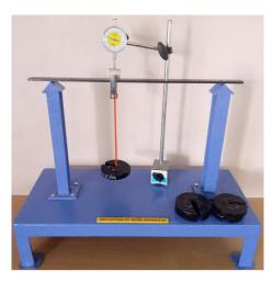
Apparatus consists of a M.S. beam with graduation scale. Supplied complete with two knife edge end supports, a hanger with knife edge and a pointer. Apparatus is supplied with a dial gauge of 25 mm travel with magnetic base and set of weights with hanger.
